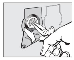
Use pointed nose pliers to withdraw the plastic filter by the bar (see illustration). Clean, put back and secure.
